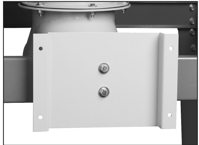
Figure 40. Model G0638 control box bracket mounted.
